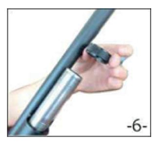
**4.**After you remove the Forearm, push "Cartridge Ramp Lock Button" and remove "Fixing Nut Barrel"
