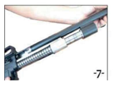
**7.**Remove the barrel to the rear slightly.
